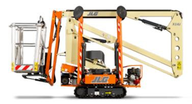
With outrigger pads removed. Pads increase width by 100 mm and height by 30 mm in stowed position.
